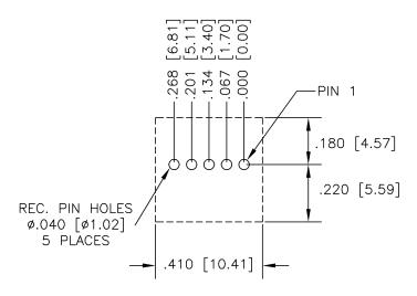
Figure 17. Recommended Footprint - Top View
