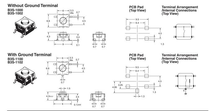
Note: Unless otherwise specified, a tolerance of ±0.3 mm applies to all dimensions. No terminal numbers are indicated on the Switches.
