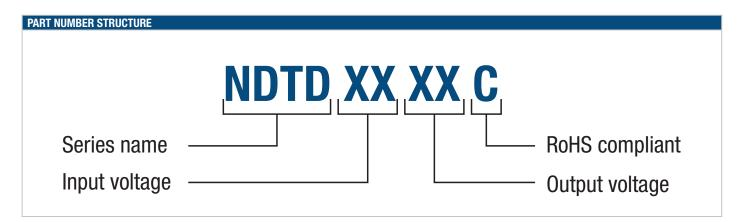
Isolated 3W Wide Input Dual Output DC-DC Converters
