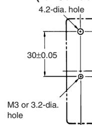
Mounting Height of Relay with Track/Surface Mounting Sockets
